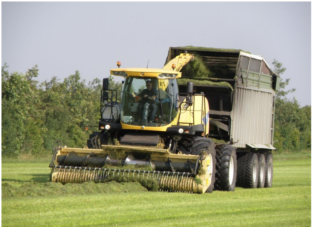
Picture 21. Forage harvester with wagon attached – both driving in the fixated tracks. There is no traffic between the fixated tracks. Usually the track width is 9 or 12 m. Photo: Mogens Kjeldal, DM&E
