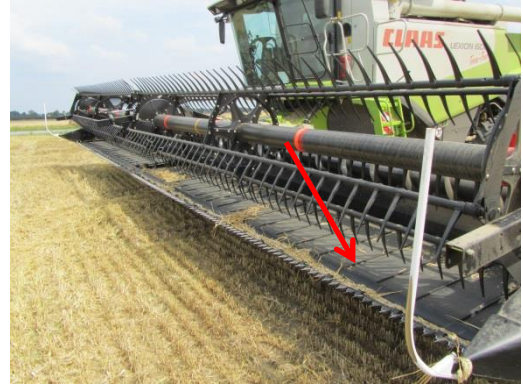
Picture 3. Draper header with belt conveyors. Photo: Henning Sjørslev Lyngvig
