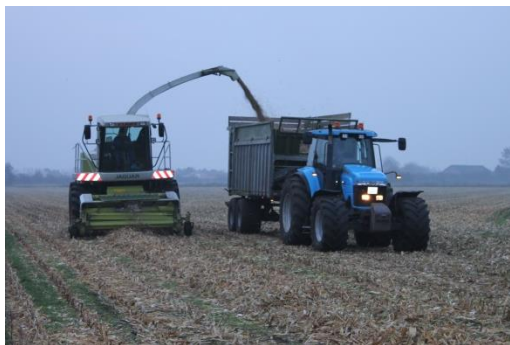
Picture 25-1 & 25-2. Harvest with a forage harvester and storage as silage was the optimal solution for maize straw concerning price and capacity. Photos: Henning Sjørslev Lyngvig
