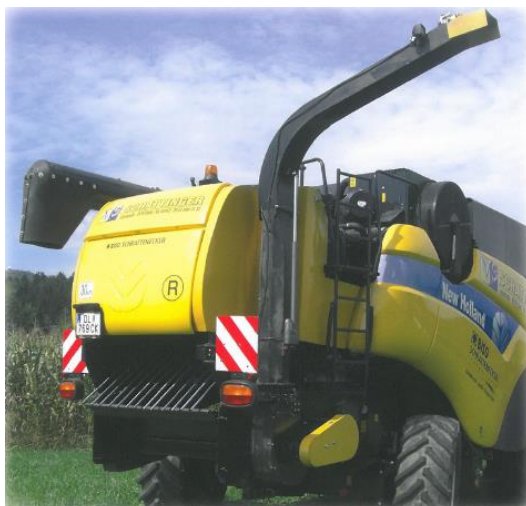
Picture 15. The threshed cobs are blown to a wagon driving beside or after the combine. Photo: BISO
