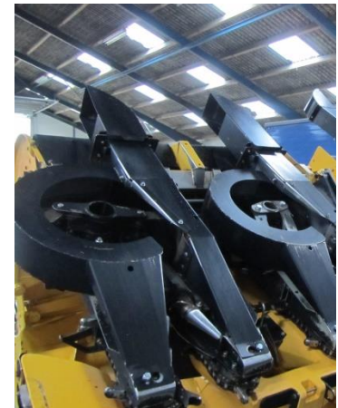
Picture 14-1 and 14-2. The stems are blown to a belt conveyor (under the yellow cover behind the header), and placed between the wheels of the combine. Photo: Cornrower / Henning Sjørsløv Lyngvig
